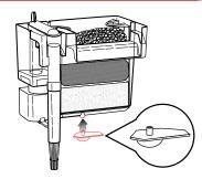
Mount power filter onto rear of aquarium and adjust leveling device by turning to required setting.
